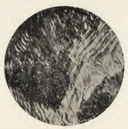
Fig. 15. Steel containing 1.24 per cent. C. Reheated to 860° C. and slowly cooled in the furnace.
